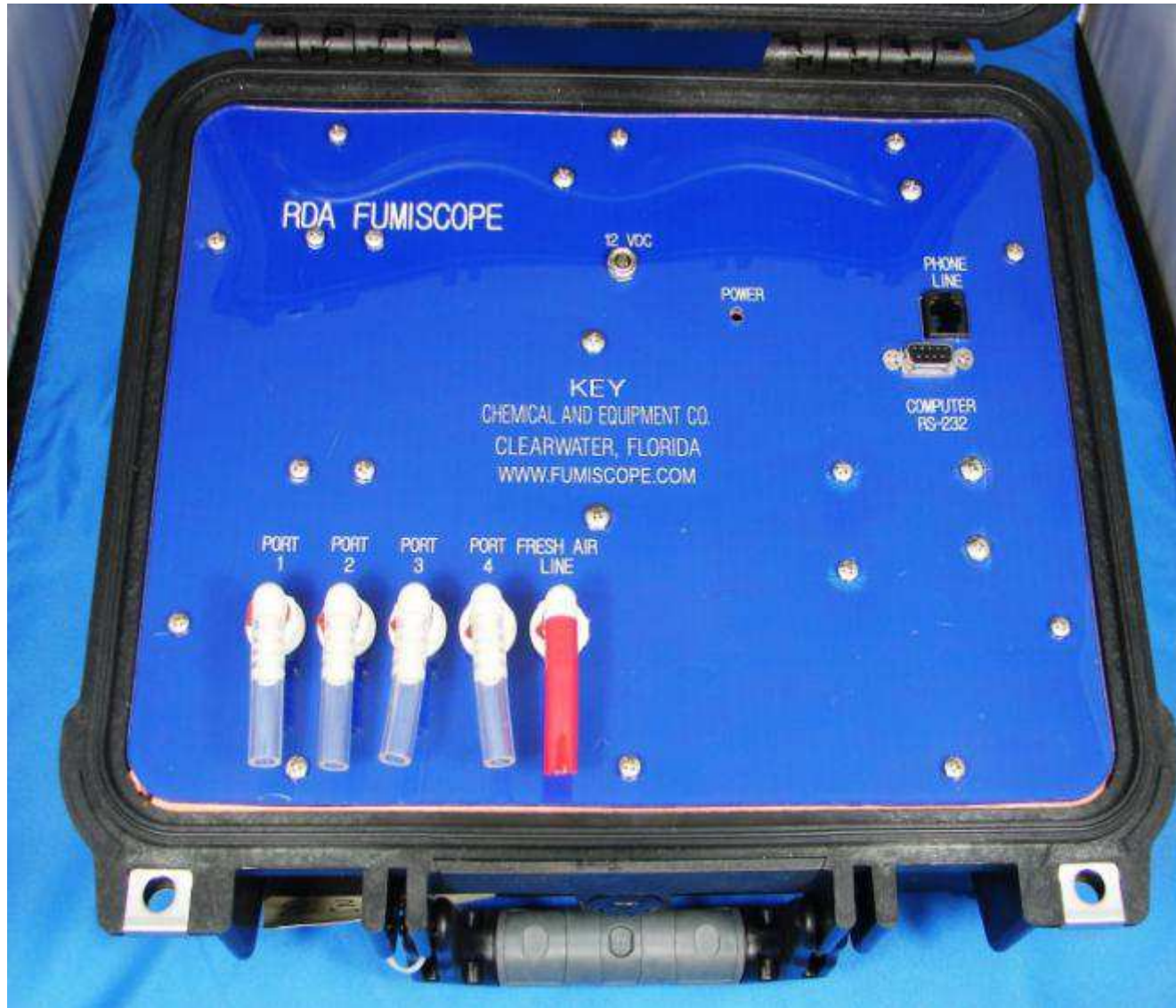
An RDA Fumiscope was also used to measure interior fumigant concentrations during fumigation and initial aeration
